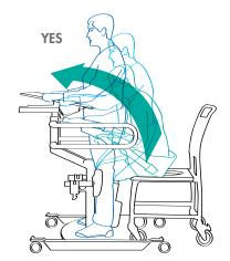
The harness lifting system has a variable geometry that ensures a relatively low compression on knee and hip joints.
