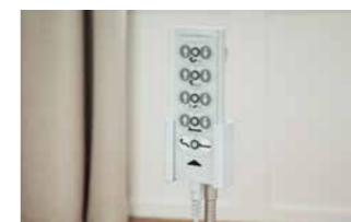
▲ Flexible transmitter holder for the handset.
